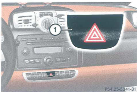
① Hazard warning light switch
