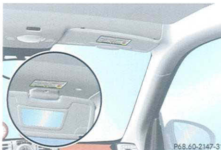
Warning adhesive label on the front passenger sun visor and the roof rail 1
