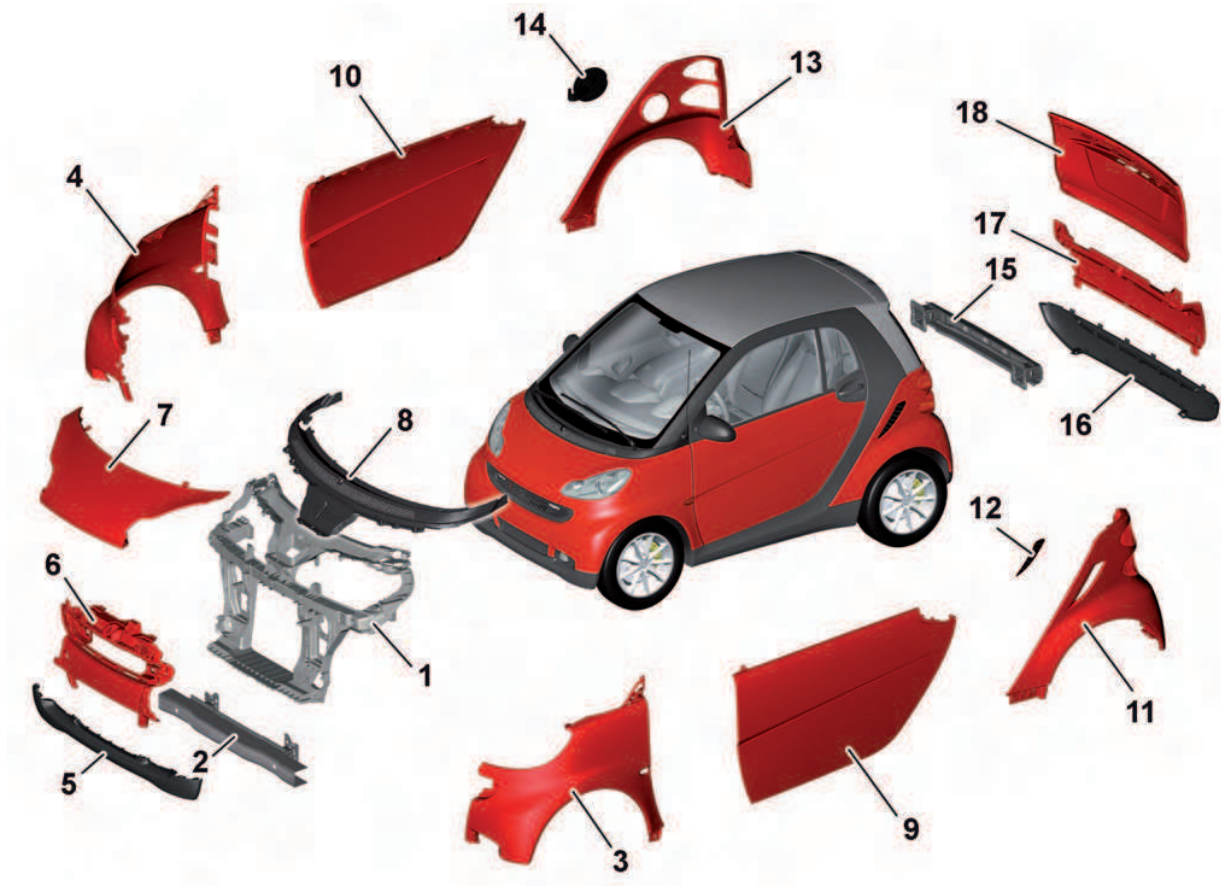
CBS components with front end module and crash management system (CMS)
