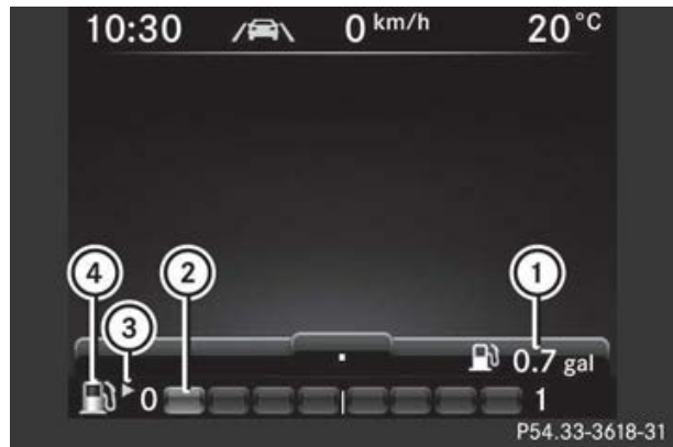
Fuel level indicator (example: colour display)
